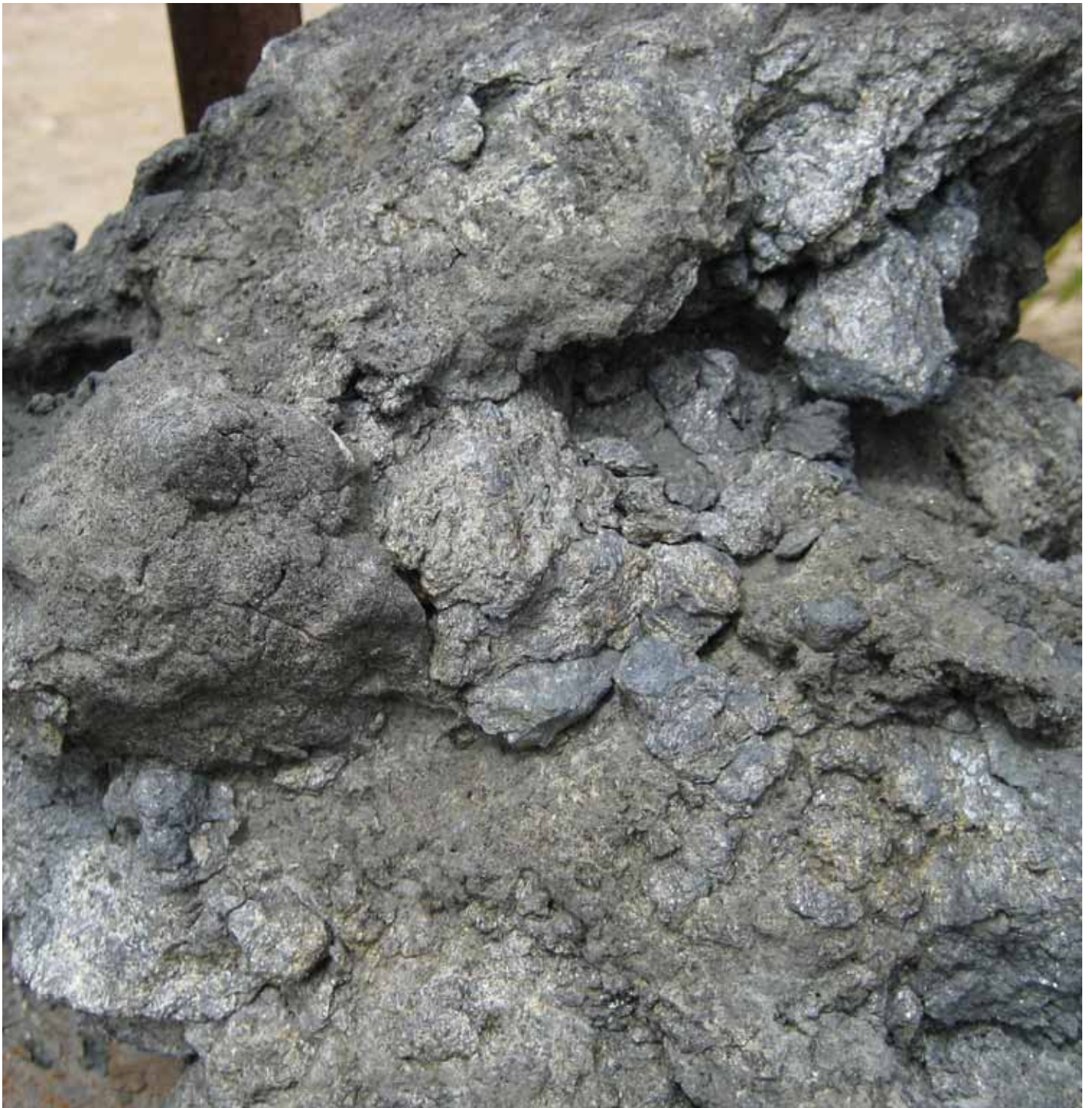
A clump of high grade graphitic ore from the Main Road deposit
